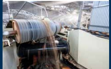
Over half a kilometre of linked conveyors and screens mechanically process mixed waste streams.
