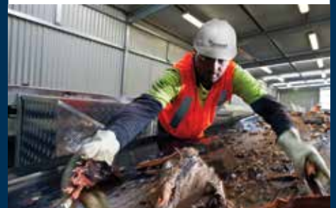
Quality control through multiple hand picking stations ensures material is separated into various storage areas.
